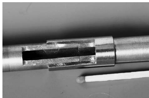
Figure 9 Two tubes connected with a coupling element prepared from the hollow cylinder.
